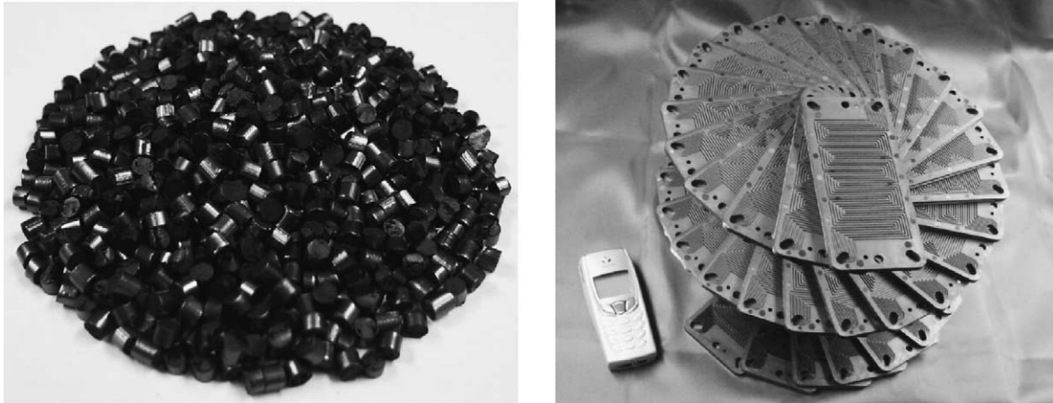
Fig. 3. Granulated compound material and injection moulded bipolar plates.
